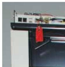
Top-mounted motor and electrical box make servicing easy
