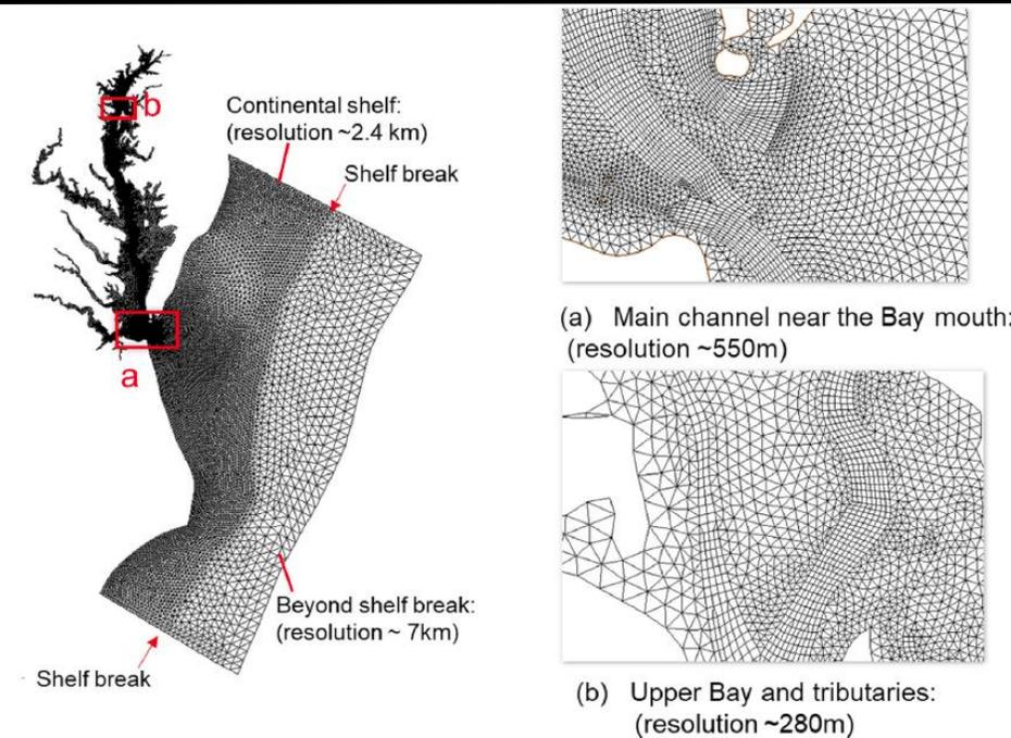
Unstructured grids (SG is a special case): flexibility in local refinement; boundary resolving/feature capturing
