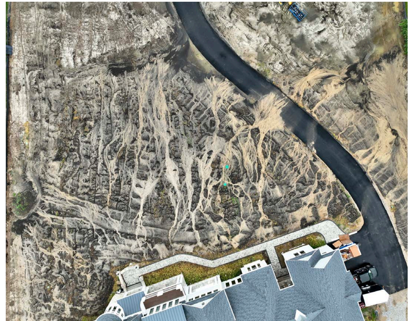
Erosion and sediment runoff from new construction. Photo credit: Driscoll Drones
